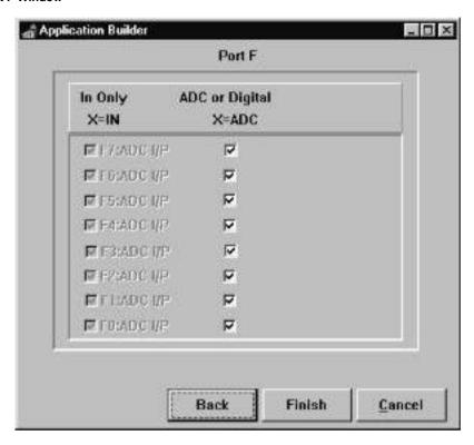
Port F is input only. Any bits not used by the ADC can be used for standard input.
