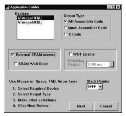
The on-board Watchdog Timer (WDT) can be enabled or disabled. If it is enabled a prescaler can be applied to lengthen the WDT time-out period. The minimum time-out period is 16 mS and the maximum is 2048 mS. If emulation is required it is recommended that the WDT is disabled.
